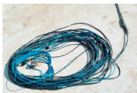
Fig. 8. MCableS - multi-point thermal passive/active measurement cable
