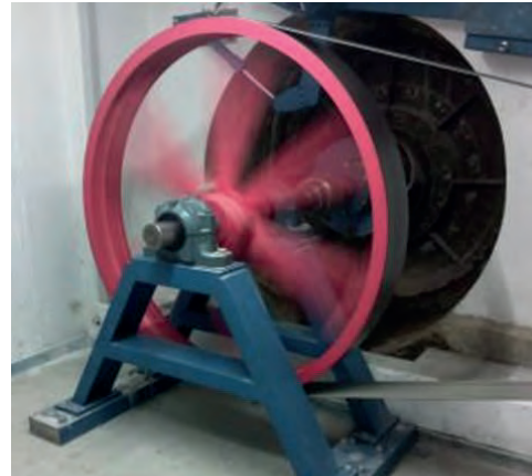
Figure 53: Flat belt drives in micro hydropower installations (Burger Wasserkraftanlagen, 2020)
