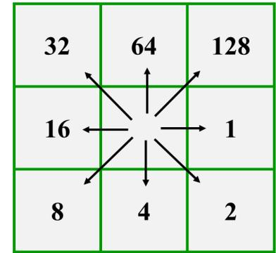
Flow direction procedure based on the D8 flow method.
